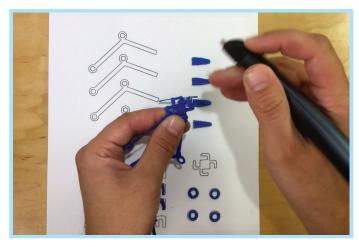
Doodle each side of the cross piece closed so that the fingers of the claw can dangle freely.
