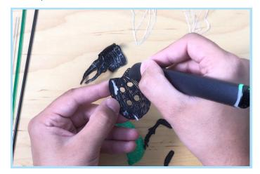
Add fresh plastic around the edges of the bottom of the body and shape it to round it out. Step 10
