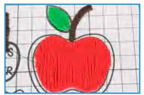
Print the stencil and fill in the PLA colours. Make sure to either use your Doodle pad or to cover the paper sheet with tape to be able to peel off the PLA afterwards!
