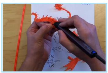
Attach feet to the back legs and legs to the body, making sure they're even and spread out a bit.
